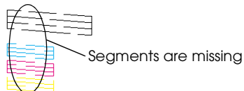
Print head needs to be cleaned.
